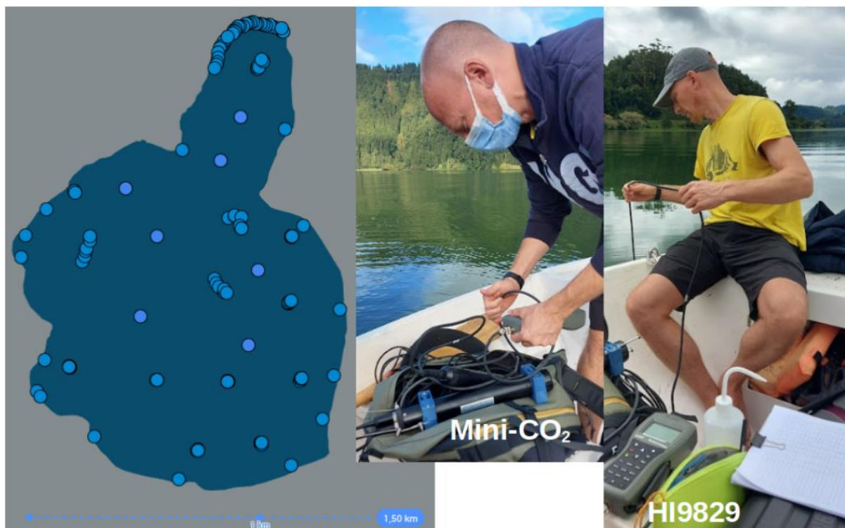
Figure 1: Map of Furnas lake (a) showing the sampling points from boat and by walk along the coast. Fieldwork photos with the Mini-CO 2 (a) and the multi-parameter (b) dropped from boat.
