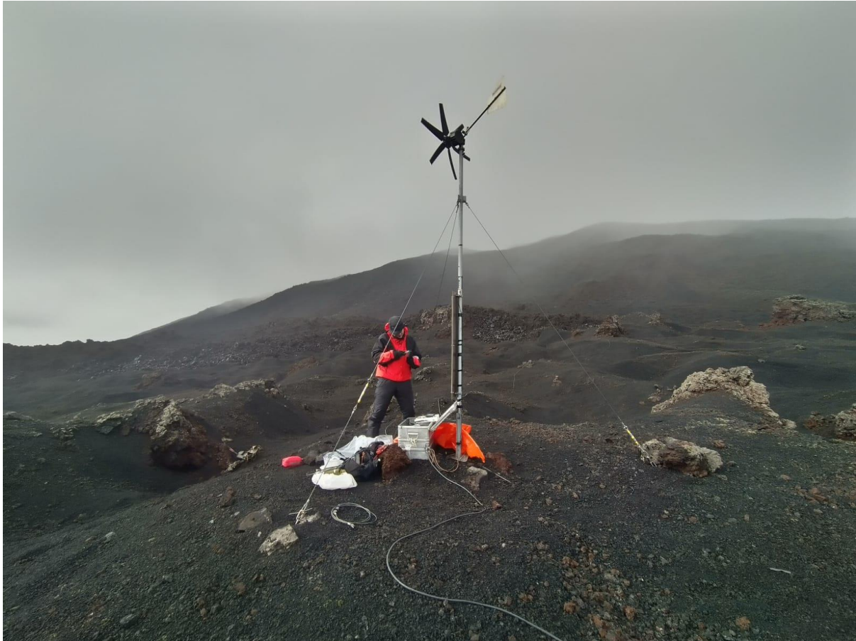
Figure 2: Servicing HERSK installation HE1 located on the eastern slope of Hekla. Martin Möllhoff stands by the pinwheel. (Photographer: Dr. David Craig).
