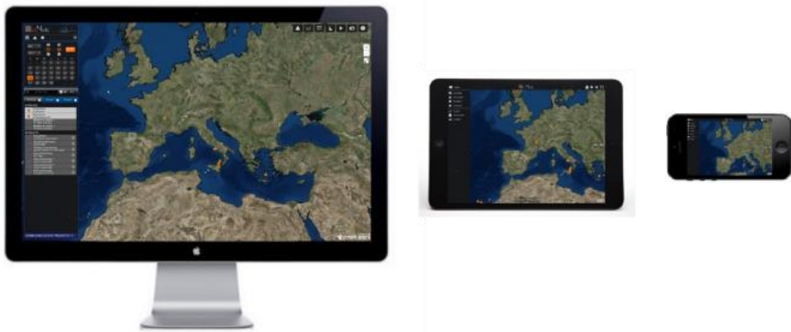
Figure 1 Open access geostationary satellite-based HOTVOLC real-time monitoring system. The system provides radiance + temperature and lava flux, ash and SO 2 concentration every 15 minutes.
